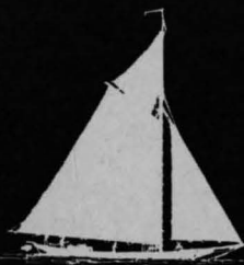
SLOOP — A small to medium-sized fore-and-aft-rigged one-masted. This is a Hudson River sloop; sloops in the coastal trade usually had smaller sail plans.
