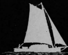
LIGHTER — A small sloop-rigged craft used for bringing cargoes to and from a vessel anchored offshore.
